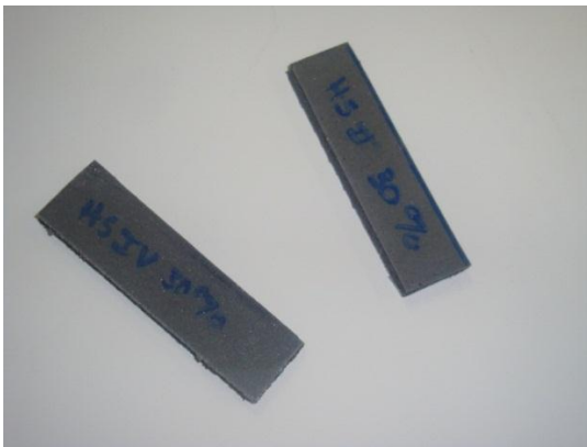
Figure 8: Image of the fabricated H-MRE samples used for experimental testing of the developed beam model.
